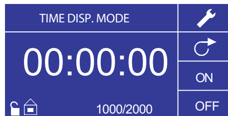
Figure 3-5. Time Dispense Mode Operation
