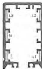
5-pole, for installations with curves
